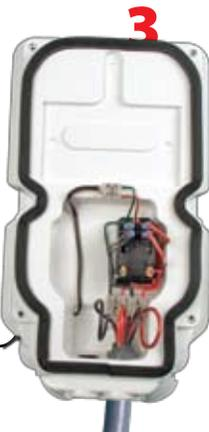
Run the brown sheathed control wire from the J-POD to your Heat Siphon and thread it through the access hole (after removing the plastic cap) and through the rubber grommet into the 3/4 inch diameter hole in the Player pocket from behind the backpanel.
